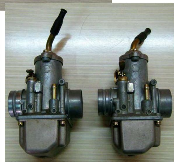
**The Jikov 2928CE is easily cleaned without dismantling the carburetor or removing the control cable, by removing the rubber hose clamps and rotating the carb upward.**
