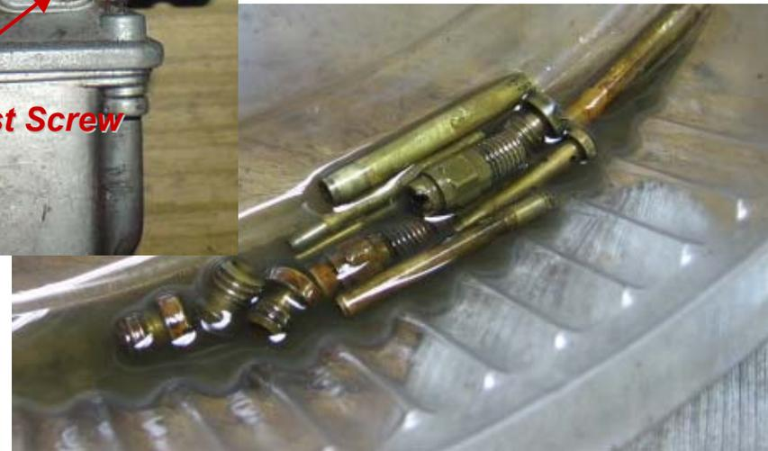
**The disassembled Jikov 2928CE is thoroughly cleaned before adjustment.**
