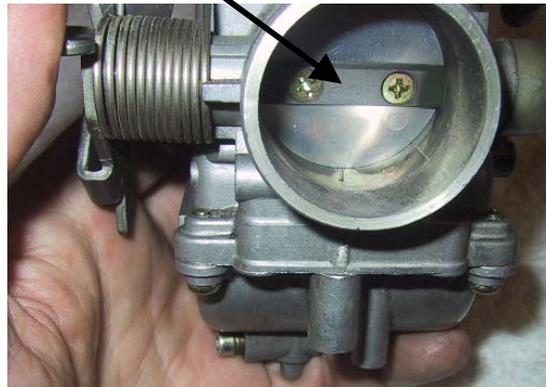
One term describing carburetors is **round-slide**, **flat-slide** or **butterfly throttle valves**.
