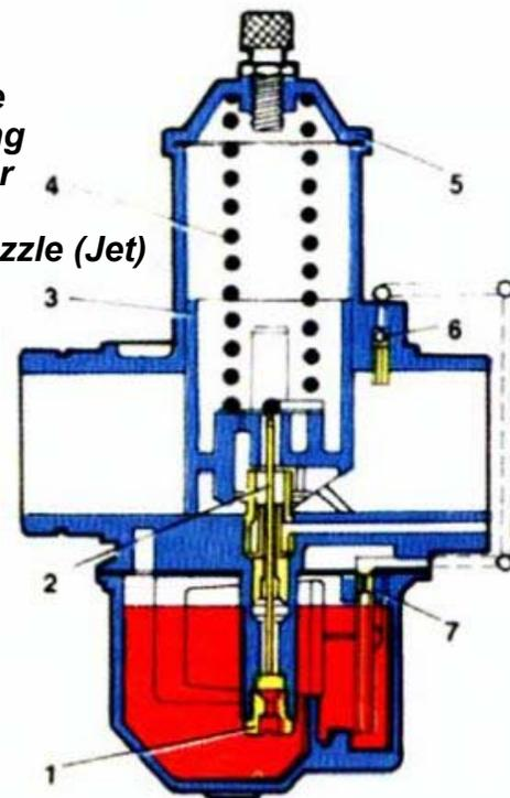
**The Jikov 2928CE carburetor has one device, never seen before; the ekonostat, serving to further enrich the mixture when lifting the throttle more than 14 mm.**
