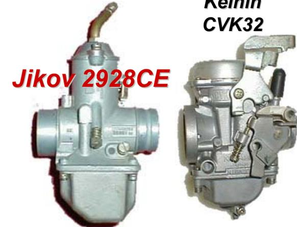
**A few Russian carburetors (L/R) were built so that the mixture-adjust screw was always on the outside, but not the Jikov 2928CE.**
